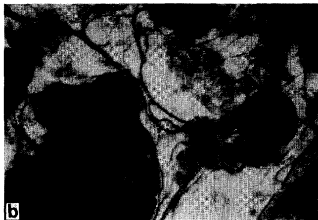
Figure 4 Photomicrograph of: (a) Polymer I, x=1.0 , taken at 232^{\circ}\text{C} , and (b) Polymer I, x=0.9 , taken at 270^{\circ}\text{C} (magnification of 320\times )
